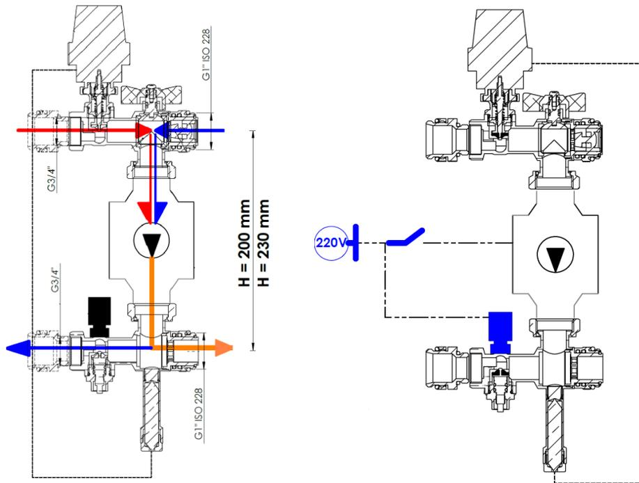
The safety thermostat is set to a temperature of 60°C. When the fluid temperature is >60°C the thermostat opens the contact, shutting off the pump.
